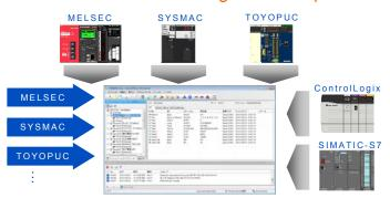
It used each kinds of OPC Server when there were some kinds of PLC in the factory. DeviceXPlorer DXP2007 series integrated all existing products and communicate with multiple PLCs. So, OPC client only access single namespace and then it can access all PLCs
